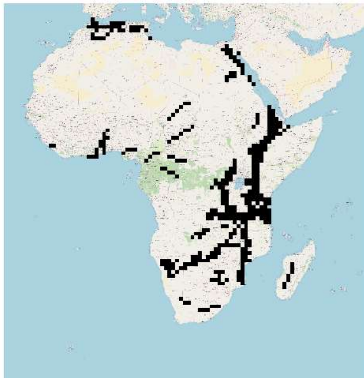
Figure 3 Active fault zone raster discretization based on location of active faults in Africa overlapping the temperature grid resolution in Figure 7
